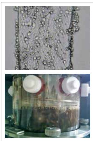
Figure 1. Growth of xylose-fermenting yeasts in bagasse fiber and fermentation of sugarcane bagasse hydrolysate in a batch bioreactor aimed at bioethanol production
