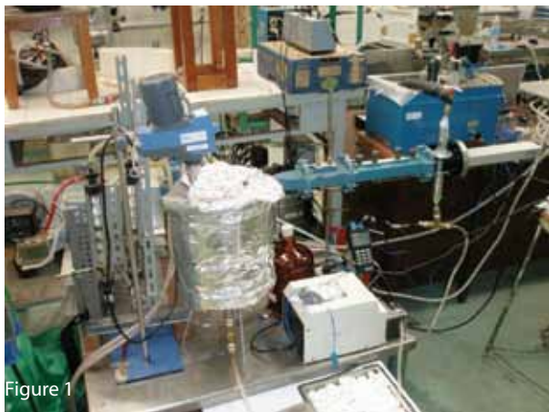
Figure 1. Assembly for continuously pasteurizing sugarcane must by using a microwave applicator. Figure 2. Assembly for studying the effect of applying US on the fermentation of pasteurized sugarcane must
