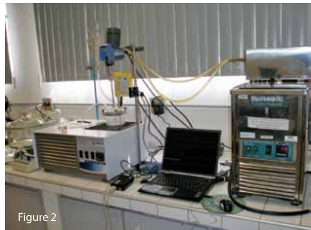
Figure 1. Assembly for continuously pasteurizing sugarcane must by using a microwave applicator. Figure 2. Assembly for studying the effect of applying US on the fermentation of pasteurized sugarcane must
