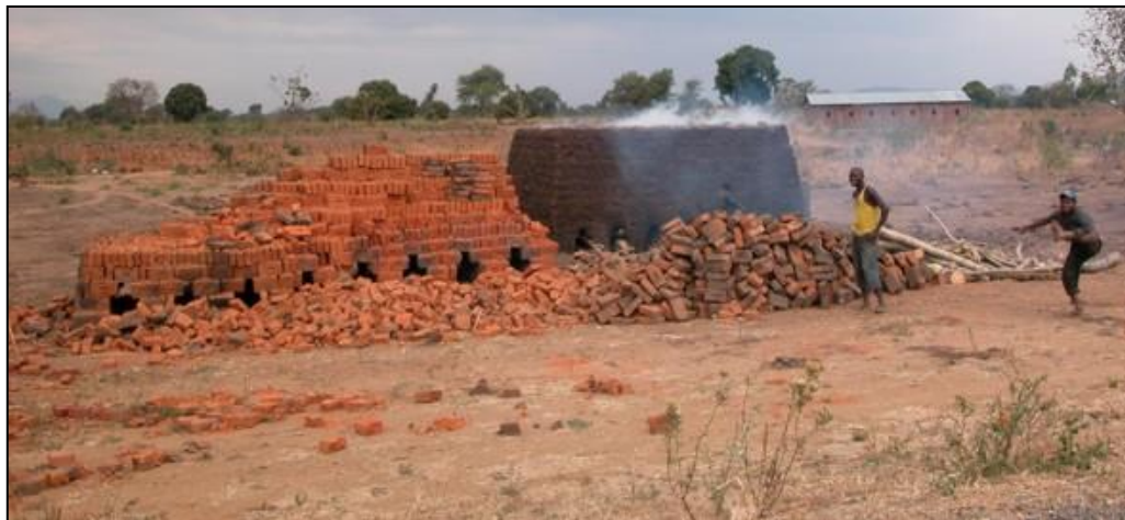
Brick-making using woody materials
