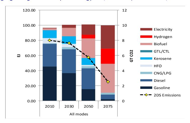
Even with H2 or batteries providing for almost all energy used in personal vehicles, busses, trains, and half of long-haul trucking, biofuels are still needed for about half of total transport energy.
