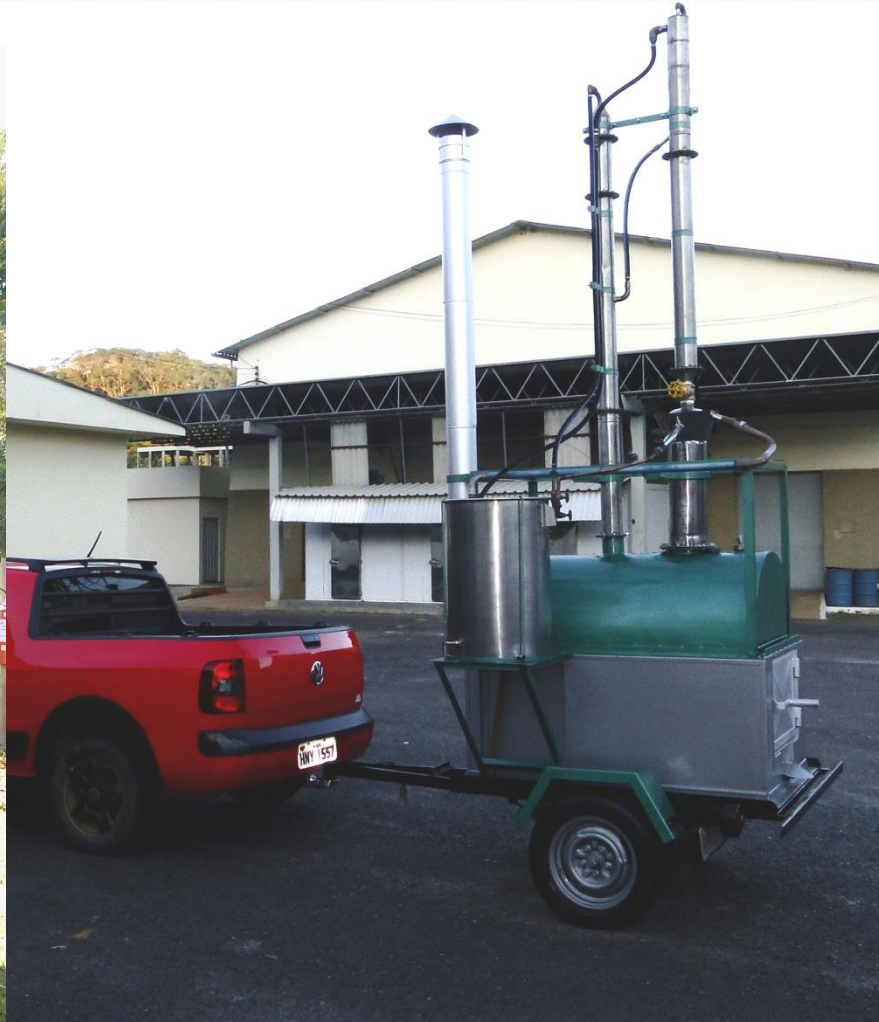
Still columns in series/parallel with direct heating furnace
