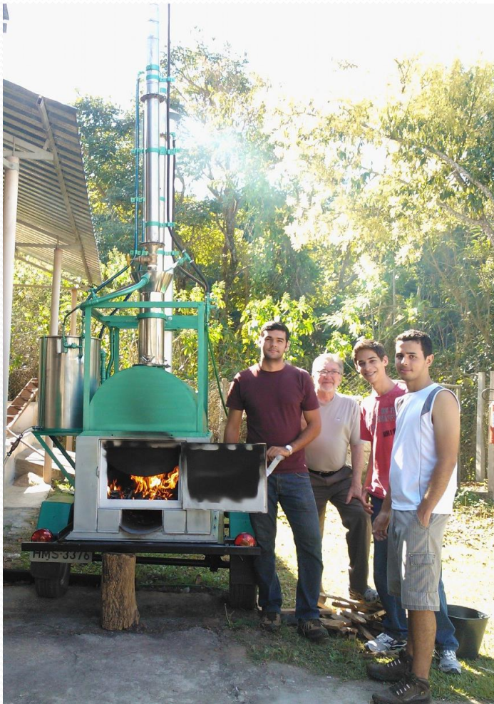
Still columns in series/parallel with direct heating furnace
